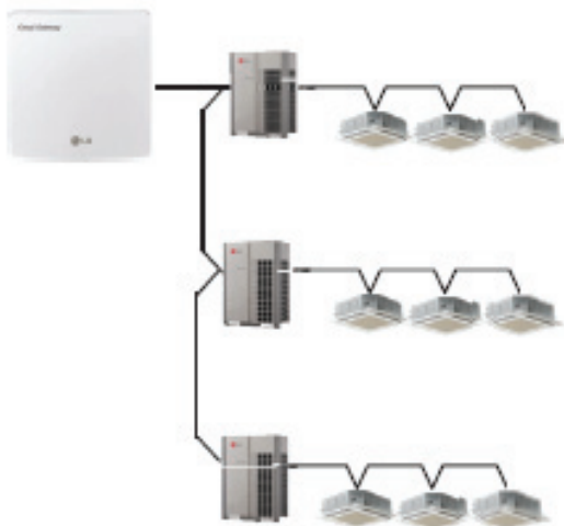
<Correct example : RS485 BUS format connection>
