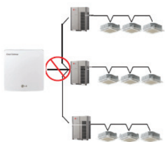
<Incorrect example : RS485 STAR format connection>
